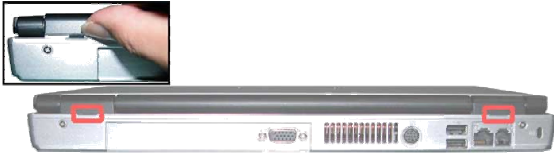
Fig. 7 Releasing the keyboard cover
